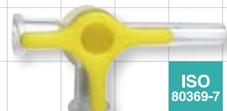
99672 2 Female Luer Locks Male Luer Slip 130 psi PC, PE
