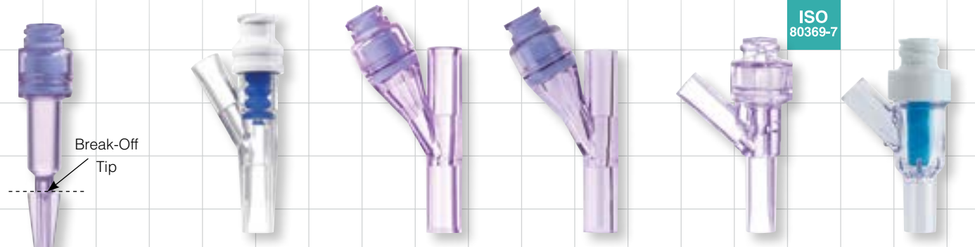
80169 Break-Off Tip Break-Off Tip Fits 0.236 inch ID Tubing (5.99 mm) PC, Silicone 91506 SmartSite™ Y Connector 0.142 inch - 0.134 inch ID (3.6 mm - 3.4 mm) Acrylic, PU, Silicone 80151 Y Connector Both Ports 0.142 inch ID (3.6 mm) PC, Silicone 80146 Y Connector Both Ports 0.16 inch - 0.11 inch ID (4.06 mm - 2.79 mm) PC, Silicone 80214 Y Connector Both Ports 0.16 inch ID (4.06 mm) PC, Silicone 91019 Y Connector Both Ports 0.164 inch ID (4.17 mm) PC, Silicone
