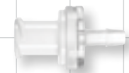
80504 Female Luer Lock Fits 3/32 inch ID Tubing (0.093 inch, 2.4 mm) 0.087 psi CP SAN, MABS, Silicone
