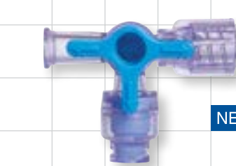
99779 Female Luer Lock Swabbable Luer-Activated Valve Male Luer Lock 1.5 psi HDPE, PC, Silicone
