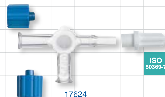
17624 2 Female Luer Locks Male Luer Slip Vented Female and Non-Vented Male Caps 0.106 inch Thru Hole (2.69 mm) 29 psi PSU, HDPE, PP
