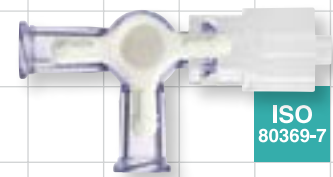
99772 2 Female Luer Locks Rotating Male Luer Lock 43 psi PC, HDPE
