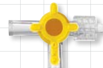
99753 90° Handle 2 Female Luer Locks Swivel Male Luer Lock 0.105 inch Thru Hole (2.66 mm) 45 psi PC, HDPE, Acrylic
